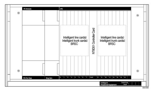
Figure 7: The NT8D37 IPE module
